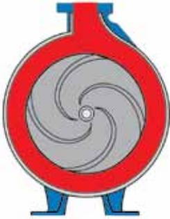
The **modified concentric volute** minimizes radial loads and distributes pressure evenly across the entire flow range for less stress and wear on components.
