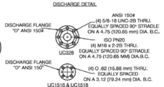
**NOTE: Drawings are for reference only. Do not use for construction purposes. Contact FTI for more detailed drawings.**
